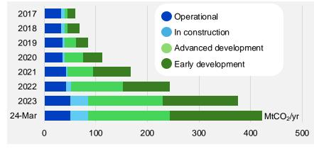
Global CO<sub>2</sub> Capture Capacity ~50 MtCO<sub>2</sub>/yr Global CO<sub>2</sub> Pipeline Capacity ~420 MtCO2/yr Data from Global CCS Institute
