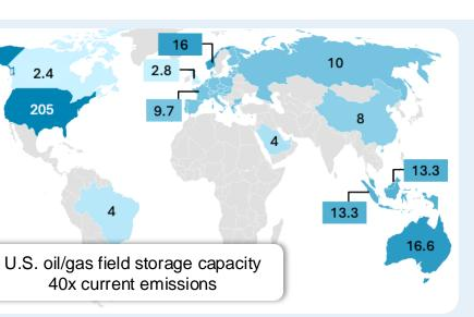
Potential CO<sub>2</sub> Storage Capacity in Oil / Gas Fields (Gton CO<sub>2</sub>) Data from Global CCS Institute
