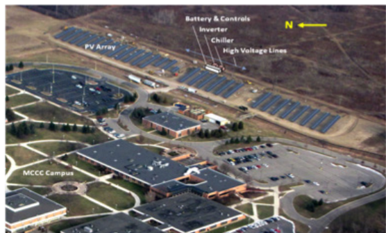
Energy Storage and 500 kW PV
