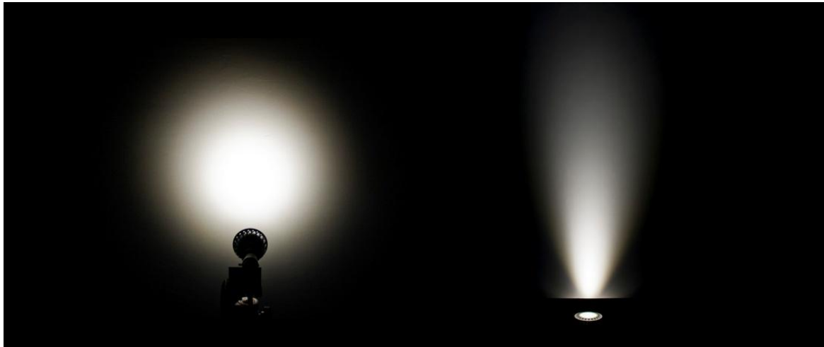
Figure 3. LED lamp beam pattern (left) and profile (right)
