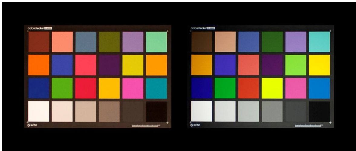
Figure 2. Identical CRI reference colors under different light sources
